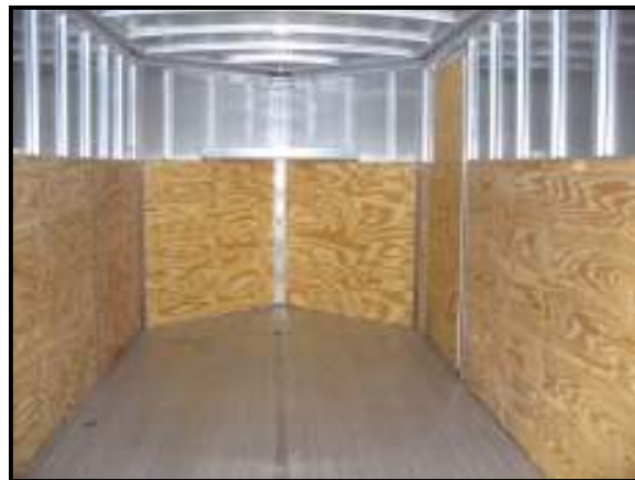
Wood Lined walls 4' high
