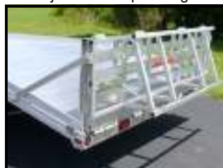
Folding ramp with spring assist
