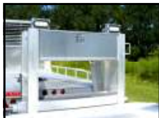
Upper GN Box & loading lights
