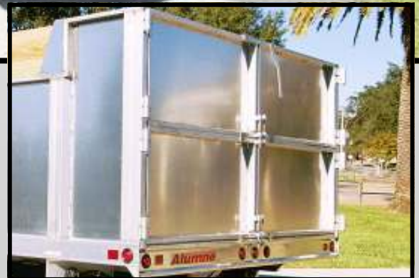
Quad Barn Doors
