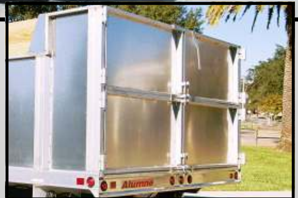
Quad Barn Doors
