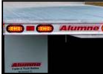
Tail mounted lights in rear apron
