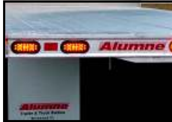
Tail mounted lights in rear apron
