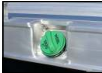
Recessed fuel fill
