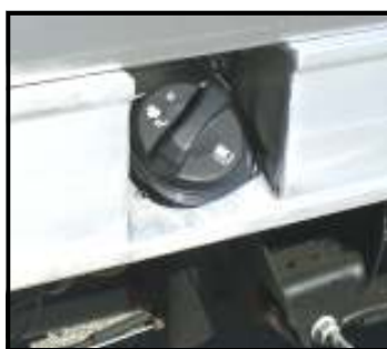
Recessed fuel fill
