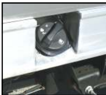
Recessed fuel fill
