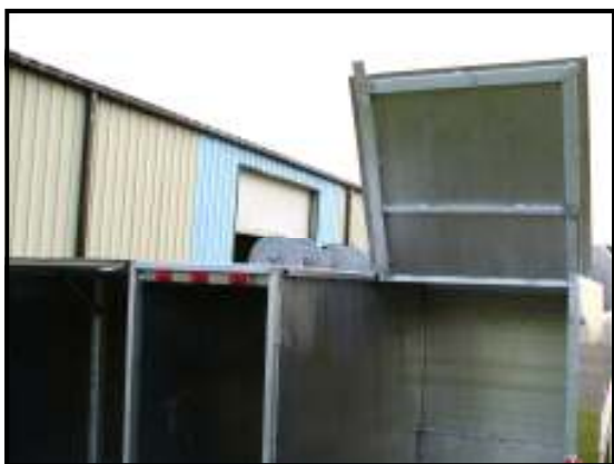
Rear spreader compartment has lid that can be raised up to allow easy access to spreaders
