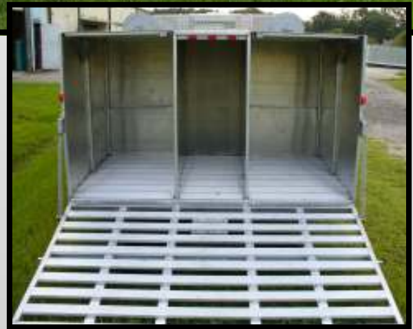
Rear spreader compartment fully enclosed for security
