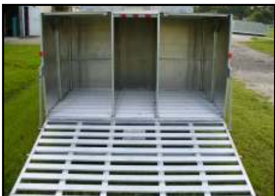
Extruded Aluminum Ramp Deck with spring assist lift
