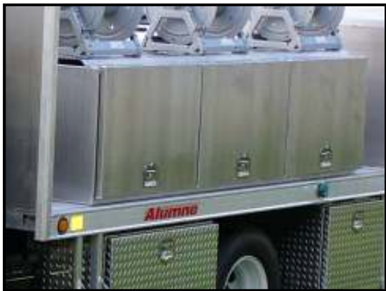
Top mounted side boxes with swing up doors for easy loading
