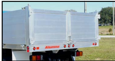
Rear barn doors
