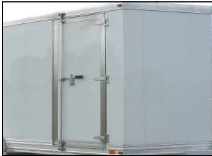
Side door with Aluminum anti-rack cam lock
